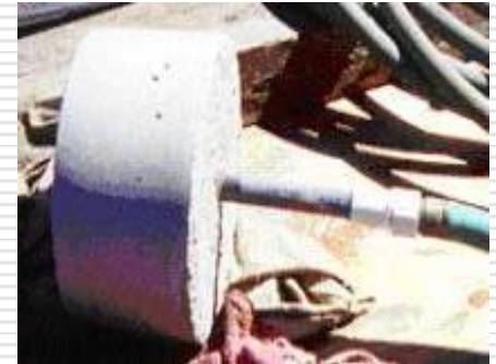
The simplest experiment was provided by our customer. They poured KF-A shotcrete mix into a pail at 1/3 its depth with inserted garden hose adapter. They kept it for 15 days under water pressure at 70 PSI or 5 Bar. Specimen was dry.
