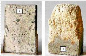
Concrete with KF-A (at left) and control specimens after 45 days in a 25% solution of Sulfuric acid treatment.
