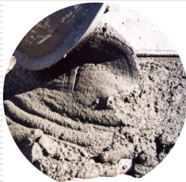
Shotcrete flow with KF-A
